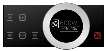
The microwave output and a default cooking time are shown in the display. The (a) field lights up red.
